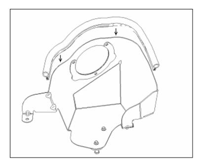
2. Install the Bellmouth (R07130019) onto the Airbox Assembly using the (3) 1/4-20 x 1/2" Button Head Screws (R18020056). Torque screws to 8 Nm. The Bellmouth should face the inside of the Airbox Assembly.
