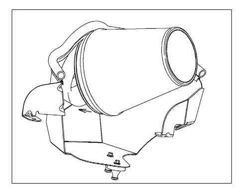
4. Install the Rubber Grommets (previously removed from the factory airbox) into the holes located beneath the Airbox, rearward of the ABS module in the inner fender well.
