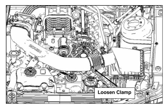
5. With a 10mm socket wrench, remove the airbox hold down bolt and set aside. This bolt will be reused later. Firmly grasp the airbox and pull up to remove it from the vehicle. Remove the two grommets from the bottom of the airbox. These will be re-used.
