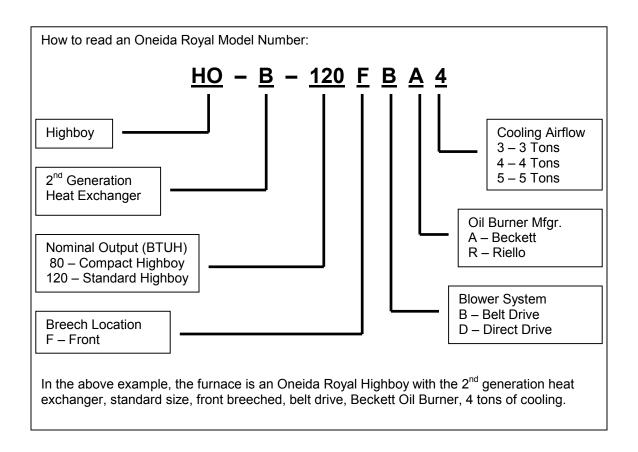
In this Installation, Operation & Maintenance Manual, the models will be abbreviated as 80F for compact models, and 120F for standard models.
