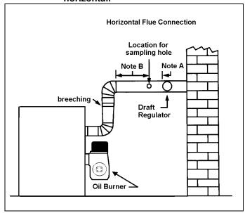
**Note A:** Locate hole at least 6 inches on the furnace side of the draft control.
