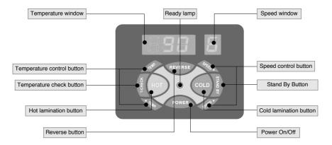
Power: It starts after pushing button, and it is set temperature 90°C and speed 6step(75mic+80g) when the start.
