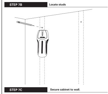
With two or more people hold the cabinet against the wall over the marked stud locations. Predrill (1) hole for a wall mount screw using 1/8" drill bit through cleat into stud. Insert one screw into stud through wood cleat.
