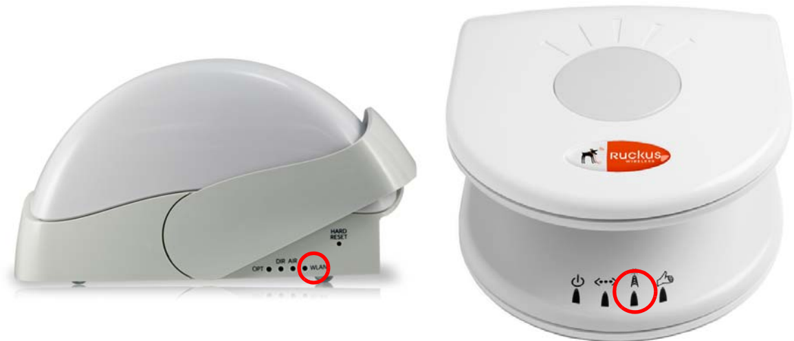
Figure 7. WLAN/Wireless Device Association LED on ZoneFlex 2942/7942 (left) and ZoneFlex 2925 (right)
