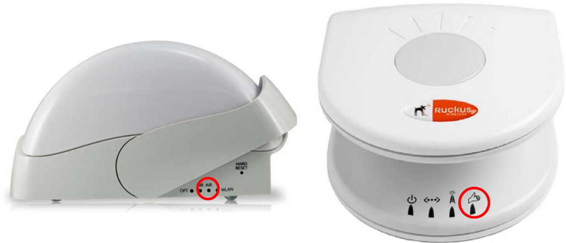
Figure 8. Air/Signal Quality LED on ZoneFlex 2942/7942 (left) and ZoneFlex 2925 (right)
