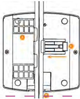
FIGURE 5 Attaching the AP and T-bar bracket with the locking tab
