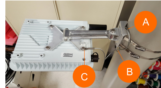
Figure 11: Attaching the security cable
