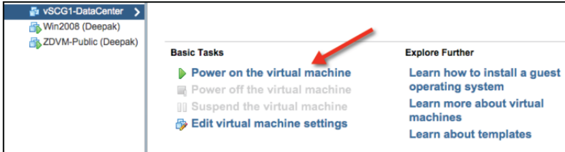
Figure 13: Click Power on the virtual machine
