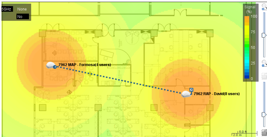
Figure 245. Dotted lines indicate that these APs are part of the wireless mesh network
