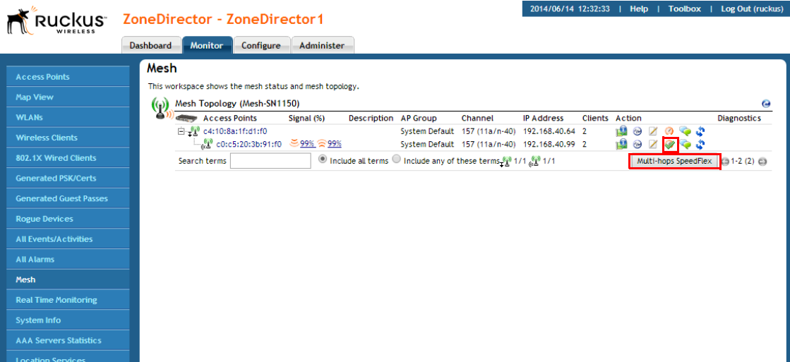
Figure 242. Multi-Hop SpeedFlex test results
