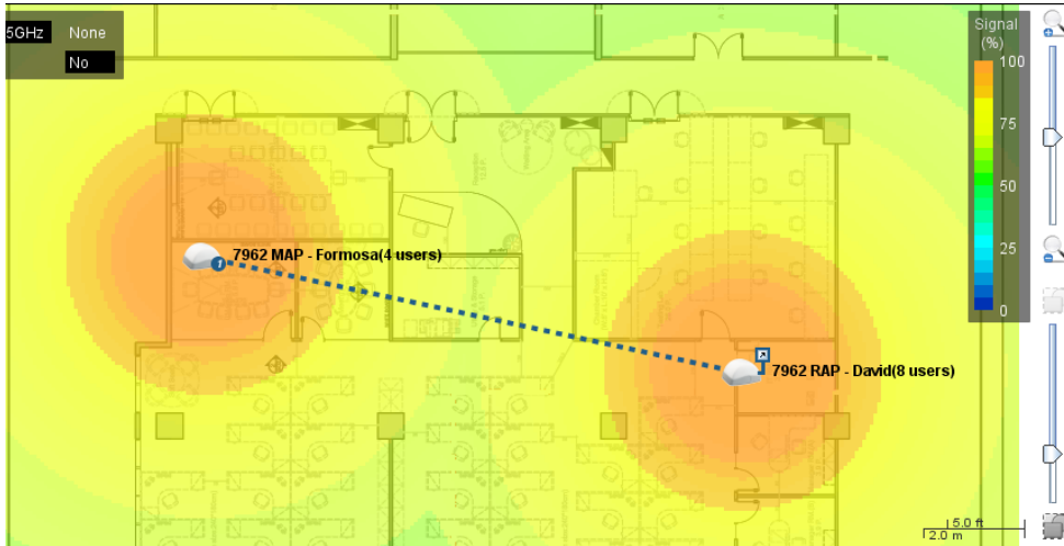
Figure 221. Dotted lines indicate that these APs are part of the wireless mesh network
