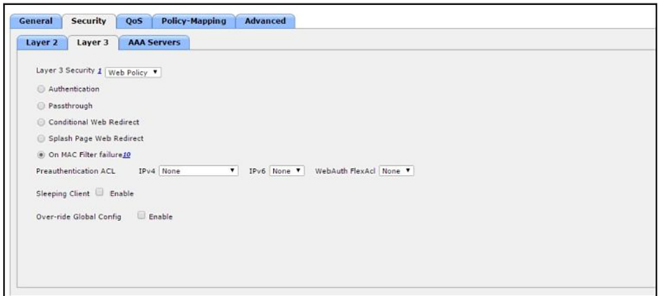
FIGURE 25 Layer 3 Settings when Using Layer 2 Mac Filtering
