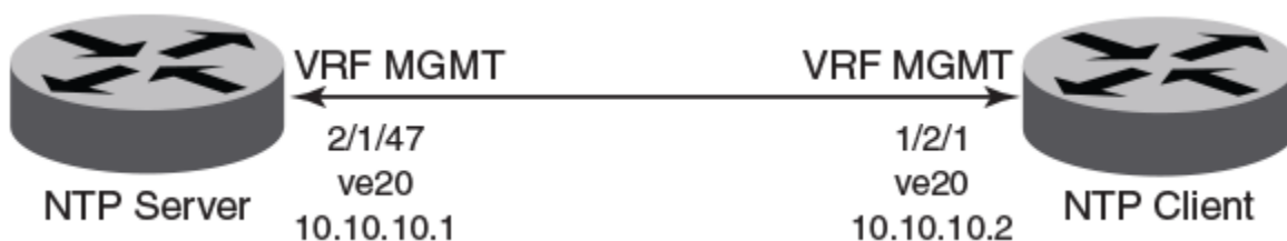
FIGURE 3 Use case 1: Management VRF forwarding with one client and one server on ve
