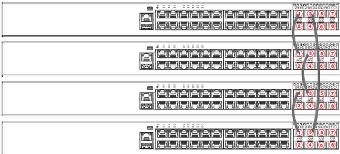
FIGURE 7 ICX 7250-24P ring stack
