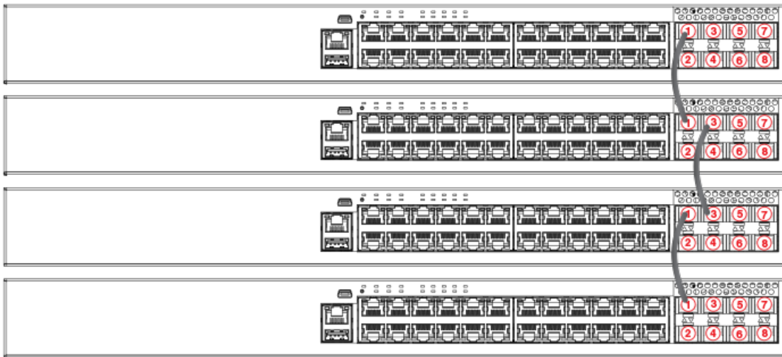
FIGURE 7 ICX 7250-24P ring stack
