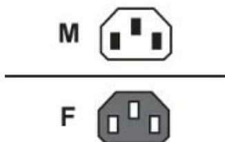
FIGURE 4 AC power cable plug and input connector
