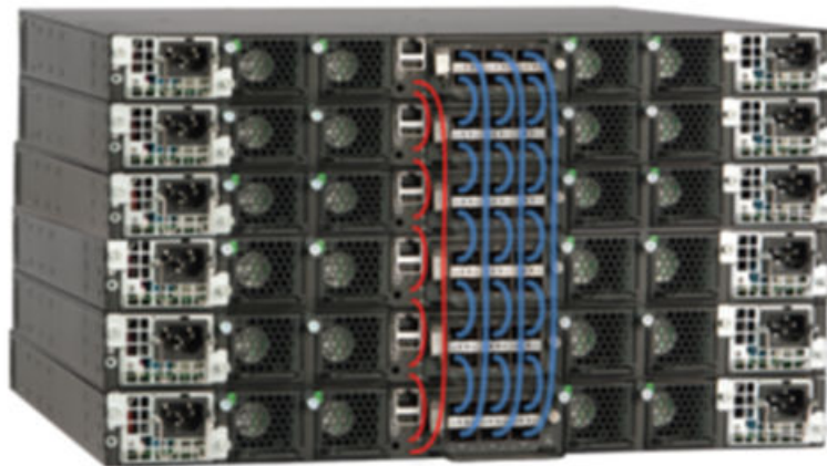
FIGURE 2 Brocade ICX 7750 Stacking Architecture
