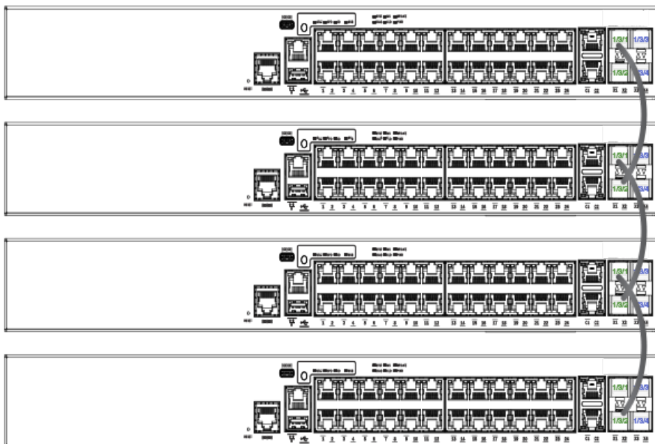
FIGURE 51 ICX 7150 24-port model, linear stack
