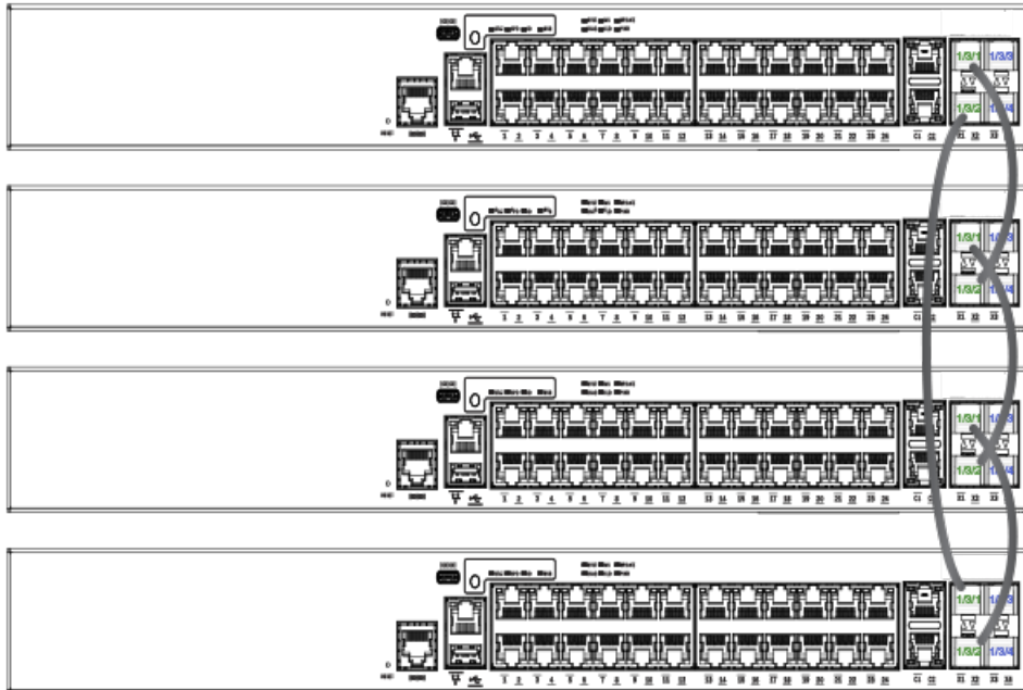
FIGURE 52 ICX 7150 24-port model, ring stack
