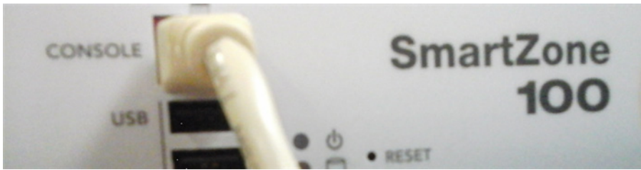
Figure 1. Location of console port
