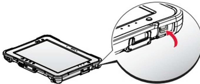
Figure 11. Closing the DC-IN Cover
