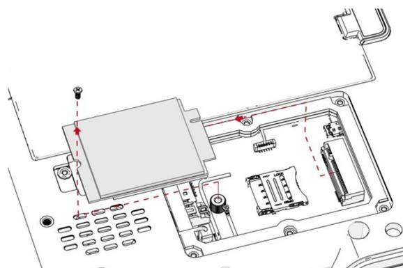
Figure 14. Back View: Remove 4G LTE card
