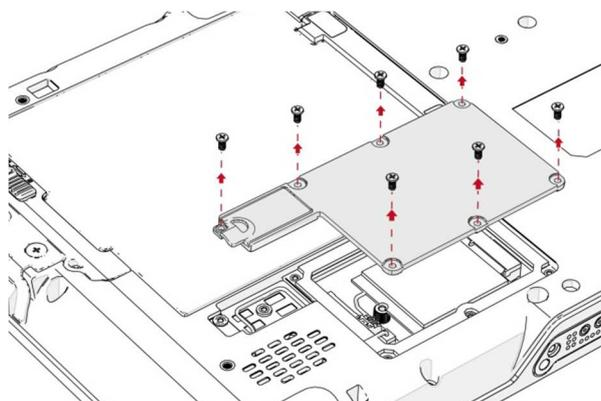
Figure 13. Back View: Remove Service Door
