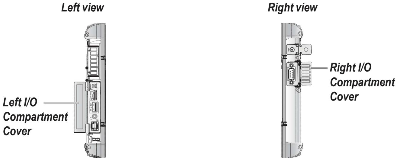
Figure 20. Side View: Locating the I/O Compartment Cover
