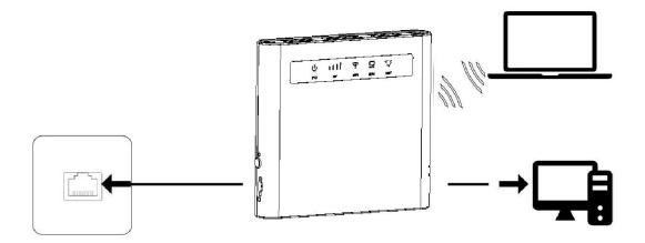
Scenario 3: Data service from Ethernet cord and VOLTE voice using a SIM card
