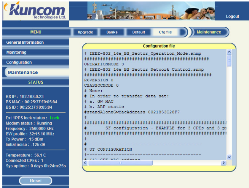
Figure 21 Maintenance – Configuration profile file screen
