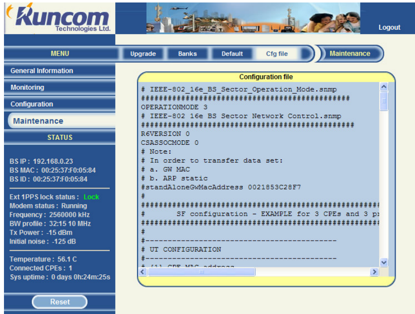
Figure 21 Maintenance – Configuration profile file screen
