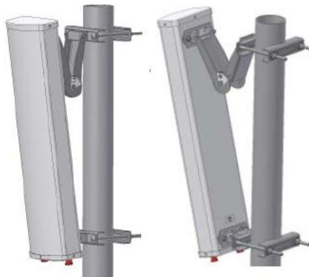
Figure 25 RF Antennas Mounting
