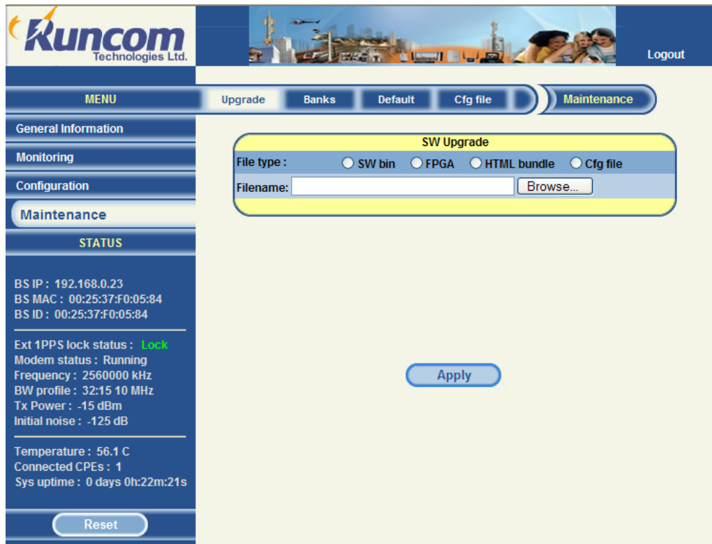
Figure 19 Maintenance Upgrade screen
