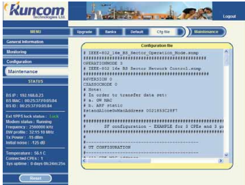
Figure 21 Maintenance – Configuration profile file screen
