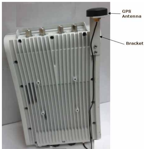
Figure 27 GPS Antenna to Bracket Connections
