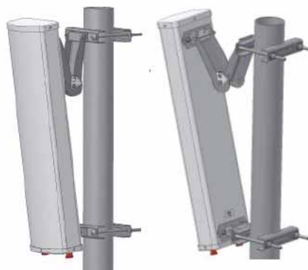
Figure 24 RF Antennas Mounting
