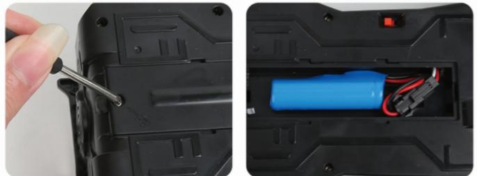
1. Loosen the screw and open the bottom battery cover.
