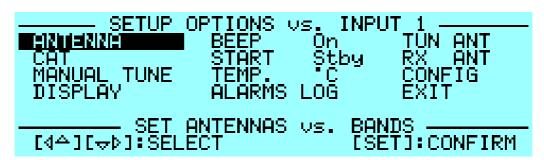
a) ANTENNA: An appropriate antenna may be assigned to each band selecting the (ANT 1, ANT 2, ANT 3, ANT 4) connector.
