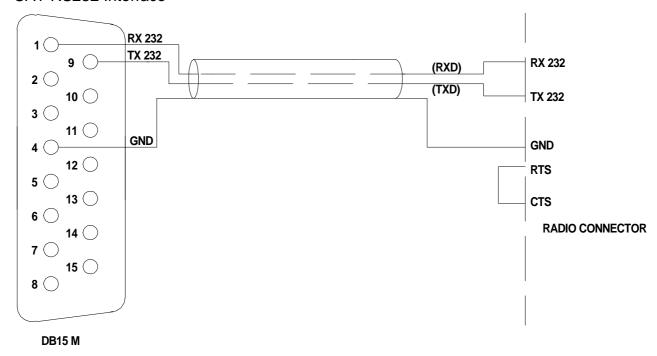
The Radio connector could be DB-9 or DB-25 male connector or female connector (read the specific manual). In the manual, also verify if the RTS-CTS link is necessary.
