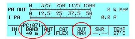
Pressing the arrow keys ( $[\blacktriangleleft \blacktriangle]$   $[\blacktriangledown \blacktriangleright]$ ) this value can be decremented/incremented until it reaches the desired value. At the completion of this operation, a time-out period (about 3 seconds) must be allowed for the "[PC=xxx]" indication to expire before another adjustment can be made.
