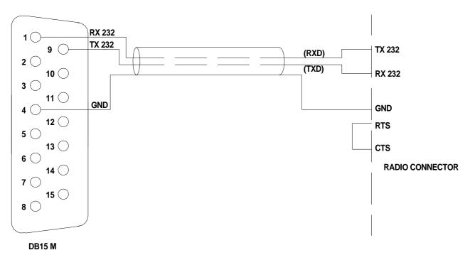
The radio connector may be a DB-9 or DB-25 male connector or female connector (read specific manual). Verify from the manual if the RTS–CTS link is required.
