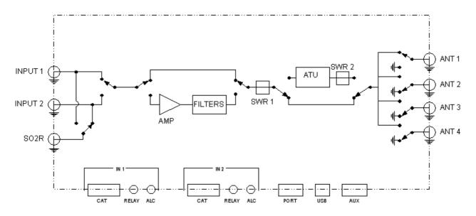
The position of the contacts, as shown in the diagram, is the situation of the linear amplifier in the OFF state.
