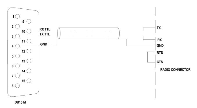
The connector is described in the transceiver's manual. Verify if the RTS–CTS link is required by the transceiver.
