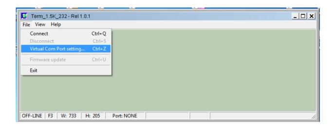
The above menu item makes it possible to access the following dialog box, which allows a direct setting of the desired **COMx** serial port for connecting to the **EXPERT 1.5K-FA**.
