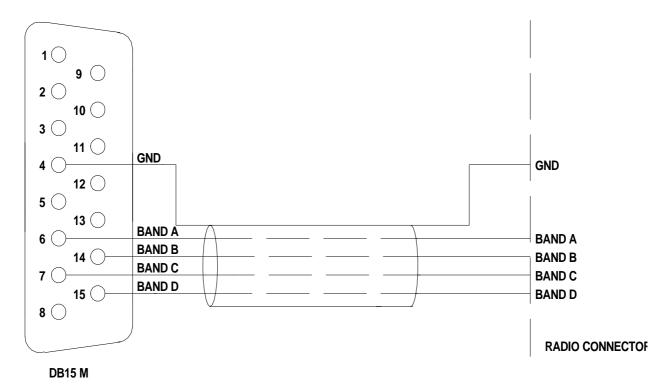
Using Band Data, instead of CAT, use the four digital signals (Band A, Band B, Band C, Band D) from the transceiver. Refer to the transceiver's manual.
