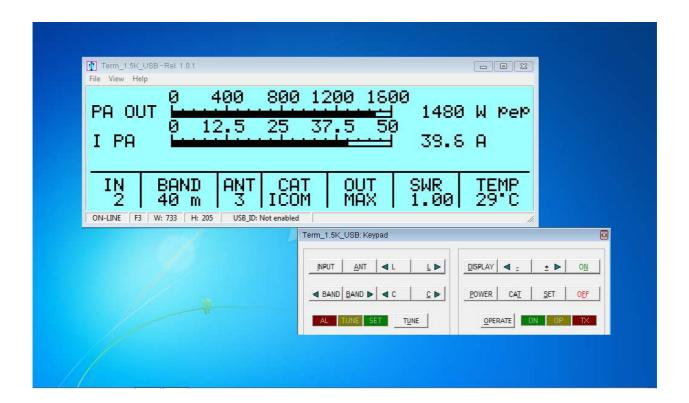
This software allows the same operation as when standing in front of the amplifier.
