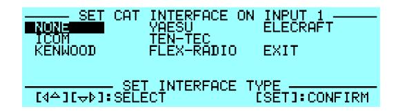
Choose the brand of transceiver or function. For the proper link wiring, see "CONNECTIONS" in this manual.
