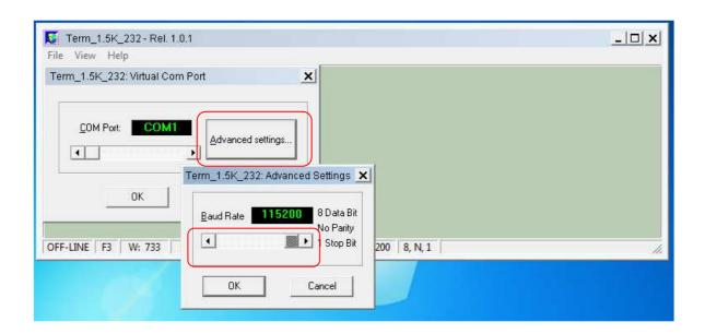
The **Baud rate** setting can be selected by using the available slider-control marked in the picture above:
