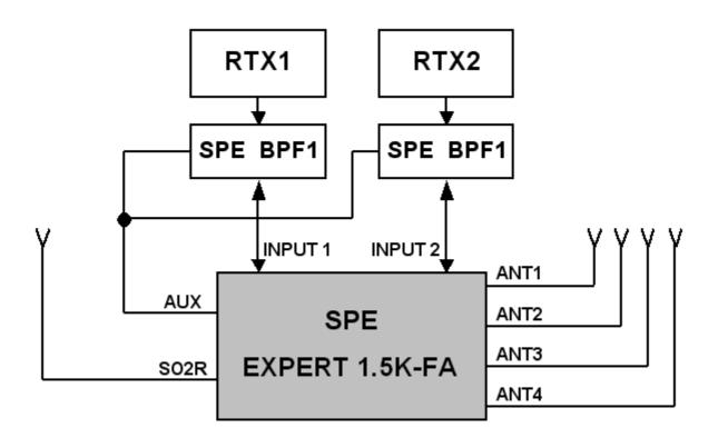
These features can be possible, as well, with the simultaneous use of the unit "SPE SO2R1, (use the AUX port with a Y cable).
