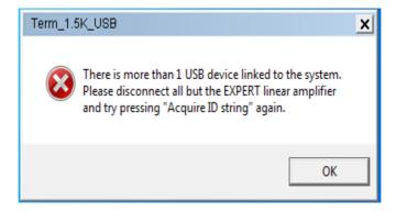
In such a case the user should disconnect all other devices except his EXPERT amplifier and to retry again using the acquisition procedure above described.
