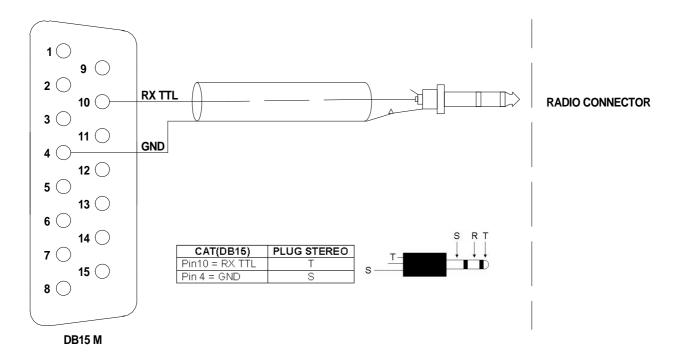
This interface is standard for all the Icom models equipped with CAT. The cable always Term\_1.5Kinates into a 3.5 mm. mono plug.
