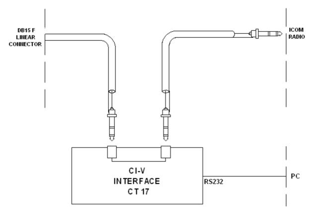
The plug from the amplifier should be connected to a CI–V port of the CT17 or similar device. The transceiver should be connected to another CI–V port.
