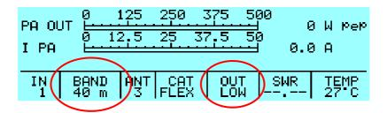
Once the correct preset has been adjusted, initiate the TX mode (RTTY, CW) to verify the output power.
