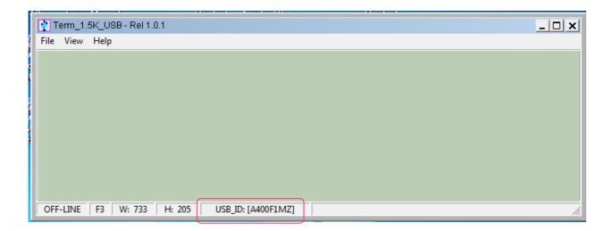
When the above described steps are completed, **Term\_1.5K\_USB,exe** will only be able to recognize and address the **EXPERT** linear amplifier whose unique **ID String** matches the one written after the **USB\_ID**: label of the picture above.
