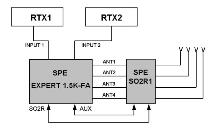
The SPE SO2R1 unit is controlled and powered from the AUX port of the 1.5K.
