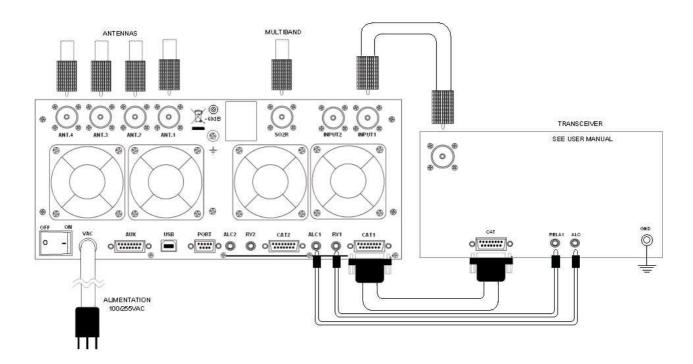
The diagram shows the connections with one transceiver only. To connect the second transceiver, repeat the same connections using the port "IN 2".
