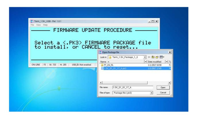
After the necessary confirmation by the user for validating the procedure, the **EXPERT 1.5K-FA** switches its display off as the updating is being transferred to the **Term 1.5K USB.exe** application
