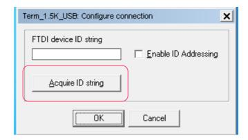
Press the <u>Acquire ID string</u> key, marked in the picture above, in order to start the <u>ID string</u> characters acquisition process across the USB data-link. This is a guided self-learning procedure. In case more than one USB communications is linked to the system, directly or indirectly thru an external USB hub, the following notification pop-up window will be shown:
