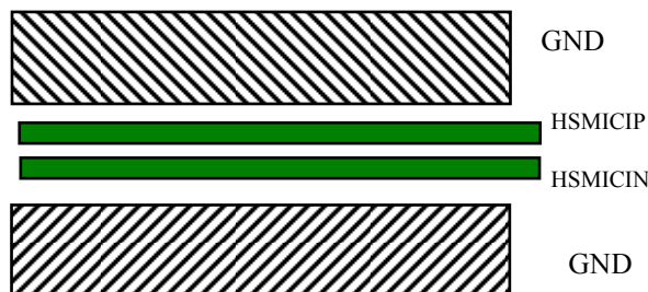
Figure 31 Layout of audio differential signals on a layer n
