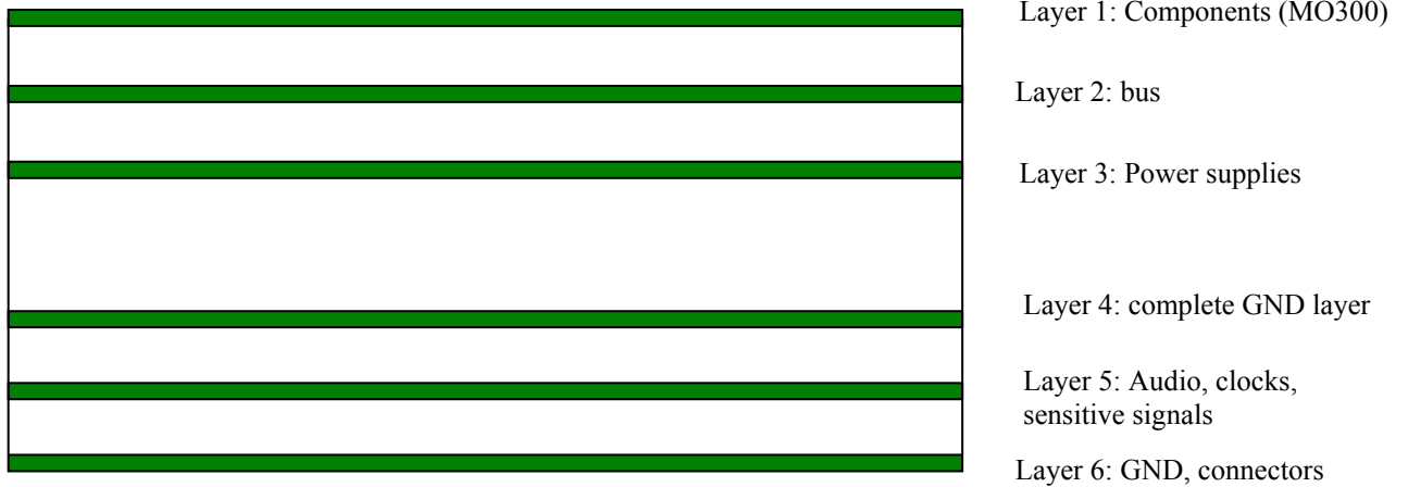
Figure 33 6 layers Stack up example
