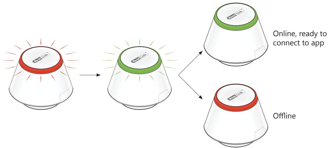
**Step 7** Once plugged in, the Wireless Internet Gateway LED light ring will flash red then green, then go either solid green (Online - connected to the internet) or solid red (Offline - not connected to the internet).
