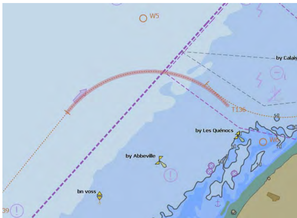
Fig. C / 9 Radius at waypoint 5 does not fit
