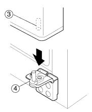
3) Insert the upper hinge shaft (⑤) into the hole (⑥). After levelling between the upper hinge hole (⑦) and the hole of the cabinet (⑧). Reattach hinge screws (⑨) and gound screw (⑩) in the clockwise direction.
