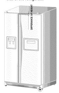
Insert a flat-blade screwdriver (-) (①) into a slot of the control lever (②), turn it clockwise and level the refrigerator.
