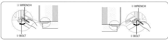
3) After adjusting the doors, turn the nut (①) turn clockwise( ) until the lower end of the bolt, then tighten the bolt again with the wrench (③) to fix the nut(①).
