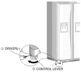
Insert a flat-blade screwdriver (-) (①) into a slot of the control lever (②), turn it clockwise and level the refrigerator.
