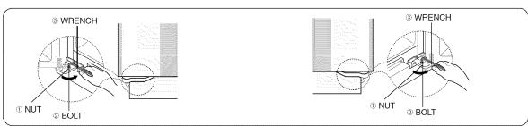
2) Please adjust the height difference between the doors turning the bolt (②) turn clockwise( ) or counter clockwise ( ).
