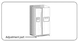
If the door of freezer is higher than that of the refrigerator.
