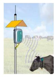
BU-500 (Base Unit) is a unit used to collect messages from tags and send them to central management system.
