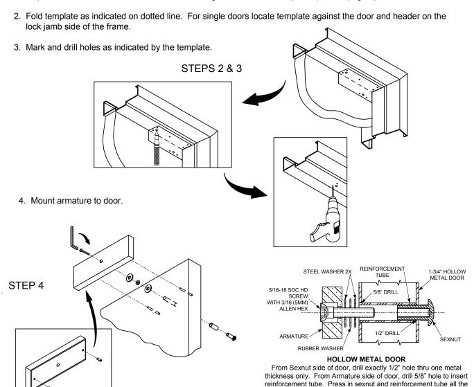
5. Install magnet onto the header with the magnetic stripes towards the door side of the stop. Assure that the magnet and armature line up properly, then tighten down <u>ALL</u> mounting screws.
