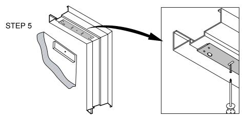
way and mount armature to door using hardware provided.
