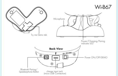
When not in use, slide Power Switch to the OFF position to save battery power.
