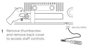
**2** Secure the attached Security Tether to a wall or other permanent surface.
