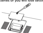
Remove pull tab from Backup Battery Compartment located on bottom of theunit.
