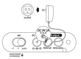
When Low Battery Icon appears on display, replace backup battery with 1 fresh CR2450 battery. Keep unit connected to DC power when replacing battery or you will lose settings.
