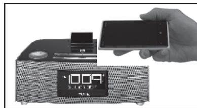
**NOTE:** To disconnect your device, simply touch it again on the NFC area of the unit. To pair a device manually, please see the following "Pairing Your Device Using Standard Bluetooth" section.
