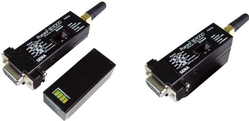
Figure 2-4 Attaching Battery Pack to Parani-SD1000
