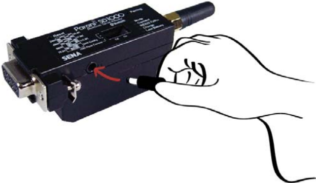
Figure 2-2 Connecting Power to Parani-SD1000
