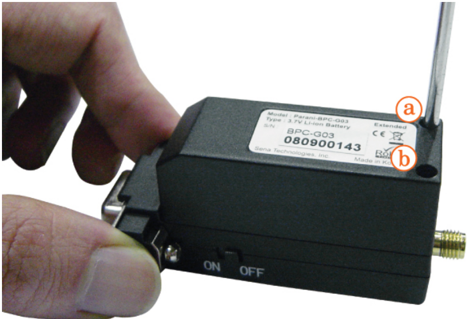
Figure 2-7 Fasten the battery pack
