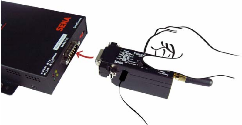
Figure 2-3 Connecting a Serial Device to Parani-SD1000
