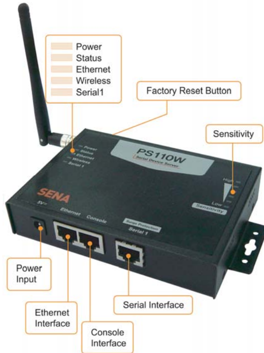
Figure 2-1 The panel layout of the PS110W
