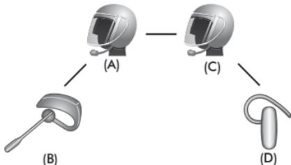
You may disconnect a four-way Universal Intercom using the same way as you do in a normal four-way intercom. Please refer to section, 15.2 “End Four-way Intercom”.
