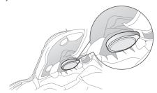
Attach the headset main unit to the clamp unit. Slide the main unit down onto the clamp unit until it clicks firmly into the bottom portion of the clamp unit.
