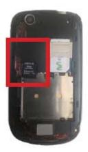
\*Note: The mobile phone does not support hot-plug function of T-FLASH in "power on" mode. Only when the mobile phone is powered off can T-FLASH be pulled out. Restart up and T-FLASH will come into effect. When using or editing files stored in the memory card, DO NOT pull out the memory card.
