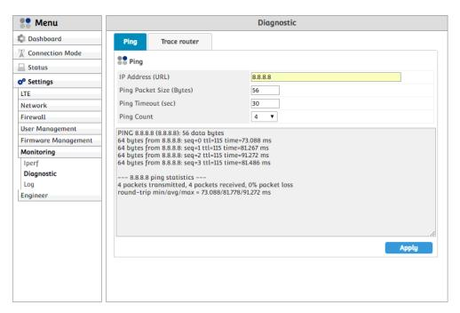
Input IP address to test, Ping Packet Size, Ping Timeout, Ping Count and click "Apply button" for starting Ping test.
