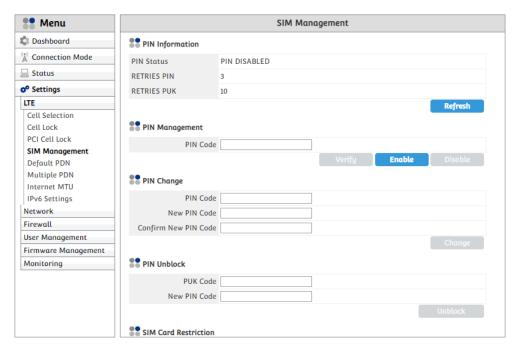
For giving higher security of using LTE, SIM (Subscriber Identification Module) can have PIN (Personal Identification Number) verification procedure. You can enable or disable SIM functionality by PIN and PUK (PIN Unblock Key).
