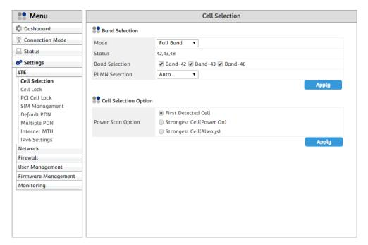
Cell Selection provides two main functions: Band Selection and Cell Selection Option.
