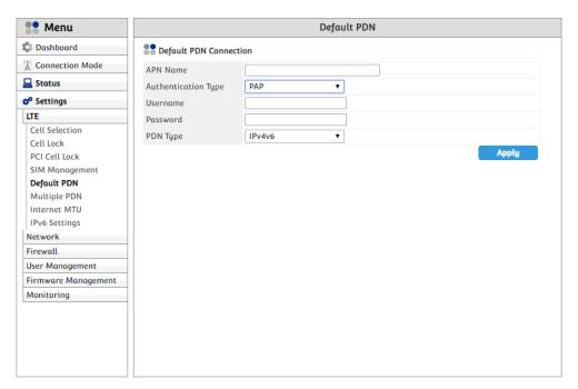
A certain network requires the device to specify "APN (Access Point Name)", "Authentication Type", and "PDN Type" for Default PDN (Packet Data Network) Connection. If these parameters are not correct, the device can't access to LTE network.
