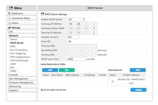
DHCP(Dynamic Host Configuration Protocol) Server assigns network configurations like IP address, Subnet Mask, and Default Gateway, to connected client devices automatically.
