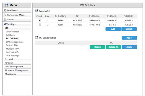
If you want the device to camp on specific cell except others, you can use this menu. The device will only try to camp on the cell in the "PCI Cell Lock List" if there is any item.
