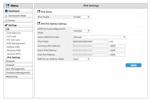
The device supports IPv6 and can be enabled or disabled by the menu. You can use IPv6 by its own purpose with DHCPv6 Auto-configuration – Stateless mode. IPv6 address is automatically assigned to its connected device. Or if you want to set IPv6 address manually (like DHCPv4), you can change the mode from Stateless to Stateful and set IPv6 Prefix, Gateway IPv6 address, and Start/End IPv6 address. Also, you can set DNS (Domain Name System) Server IPv6 Address manually.
