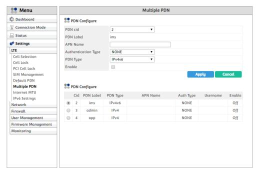
By default, the device is set as Default PDN (Packet Data Network) for LTE registration and PDN Connectivity. But if network requires Multiple PDN for using "internet", "IMS (IP Multimedia Subsystem)" or any other purpose, you should set and enable Multiple PDN function by this menu.
