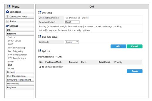
QoS(Quality of Service) is used for maximize its usage of limited bandwidth, and optimize its load. This function can allocate minimum or maximum bandwidth to those PCs connected. So, in case that one PC occupies too much bandwidth load, QoS can control that PC's bandwidth and minimize its influence to others for seamless internet environment.
