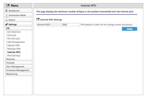
In case that LTE network requires the device to limit MTU (Maximum Transmission Unit) size, you can set in this menu. Change of MTU size is usually for IP packet management between LTE network entities. Normally, the default value, 1500 is used without any problem.
