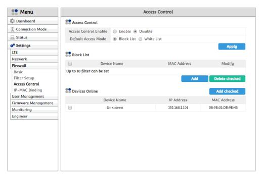
"Access Control" function can control the device (PC, Smartphone, etc.) accessibility to CPE by management of "White List" that is list of access granted to CPE, and "Black List" that is blocked to access CPE. In case that "White List" is set, only those devices in the list can access to CPE. Otherwise, "Black List" is set, those devices can't access to CPE. "White List" and "Black List" can't be used at the same time. Only one "List" is available at one time.
