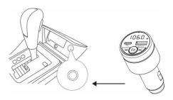
2. The product will automatically power on after insert and display HI--Voltage--FM frequency 3. Turn on your car FM radio, and choose the blank
