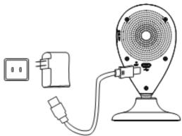
Connect the power supply with the IP Camera, then the bluelight will be on, after 2 secondsthe red lightis always on.
