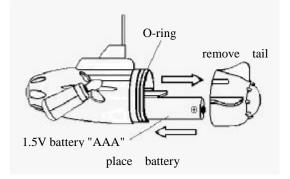
2. Install the "tail cover" back to the submarine (please do not loose the two water-proof "black O-ring, or the water will get in). When the upper and lower cover is in tight fit, the baseline must be aligned, and the power will start to receive signal. The power will automatically shut down when the "tail cover" is removed.
