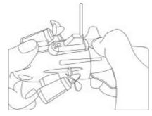
Caution: When opening the tail cover, do not apply force on the tail wing to avoid the possible breakup.
