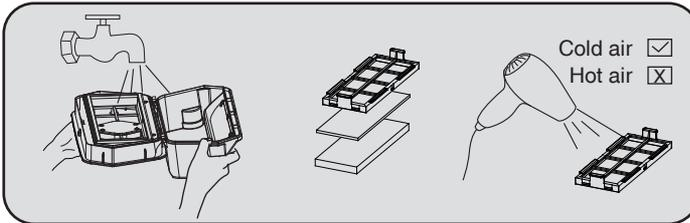
4. The dust box can be washed with running water. (Note: the dust box should be completely air-dried before re-inserting)
