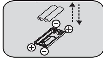
2. Place two AAA (#7) batteries into the compartment.
