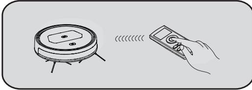
3. After installing the battery, turn on the power switch of the cleaner. Check whether the remote control can control the cleaner. In case of no reaction, refer to Recoding the Remote Control Code on Page 12.
