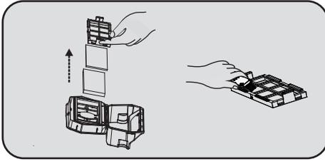
3. After take out the filter, wipe off the dust with the cleaning brush.
