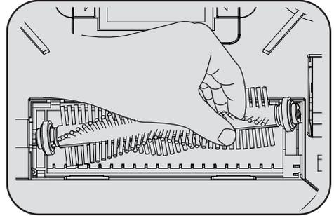
2. Clutch the main brush and lift it upward.
