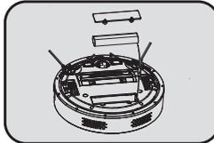
Switch off the cleaner when taking out the battery.
