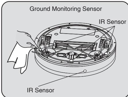
After each cleaning work is completed, dry cotton cloth is used to dry the transparent plate to prevent dust from being accumulated on the plate so as to affect the performance of this product.
