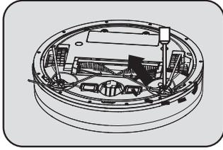
1. Unscrew the screws on the side brush with a screwdriver.
