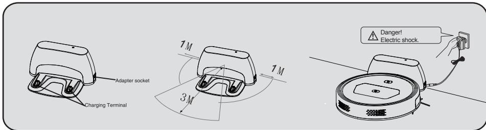
1. Place the charging base on the flat ground that is perpendicular to the wall. There is no obstacle within the range of 3 meters in length and 1 meter in width. Press the charging base with force to make it more firmly pasted on the floor. After plugging in the adapter, insert the DC plug into the DC port.
