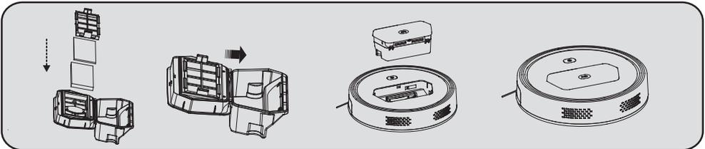
5. After cleaning, re-assemble the filter in the dustbin first, and then, insert the dustbin into the cleaner.
