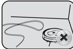
Clean up the wires and sundries on the ground in case of being tangled into wheels and brushes.
