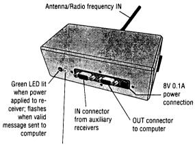
Amber LED flashes when message received at receiver antenna.
