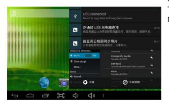
Press "USB connected", select "Turn on USB storage". The device is recognized at Explorer of the computer. Now you can use it as an external storage.
