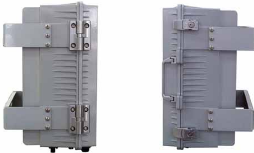
< Fig. 4 > Side View of CDMA Repeater
