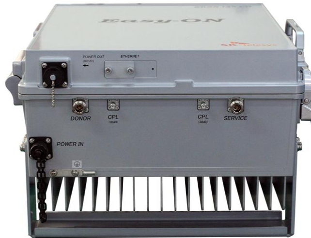
< Fig. 5 >Bottom View of CDMA Repeater
