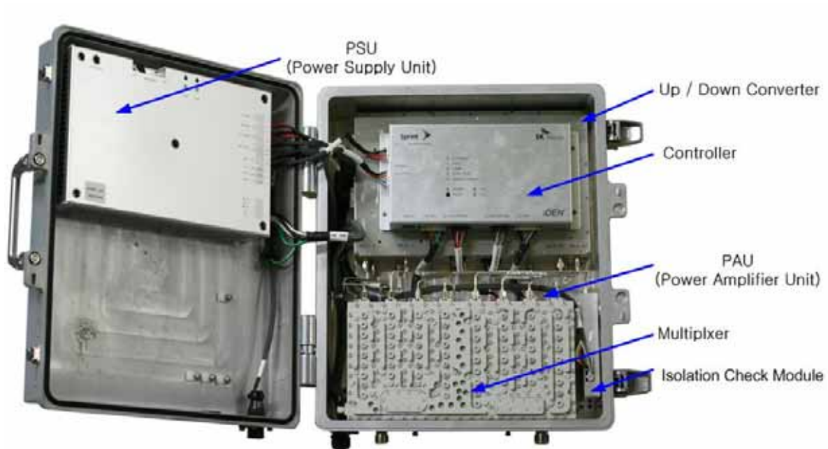
< Fig. 9 > Internal Construction of iDEN Repeater
