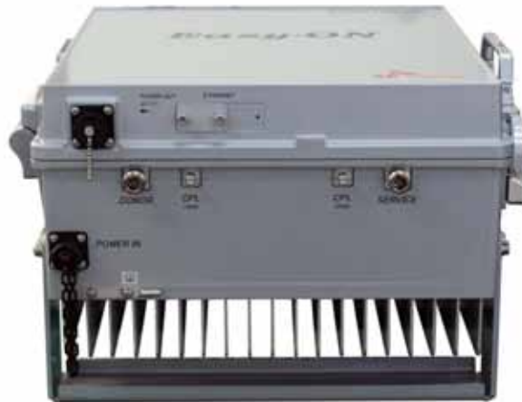
< Fig. 5 > Bottom View of iDEN Repeater
